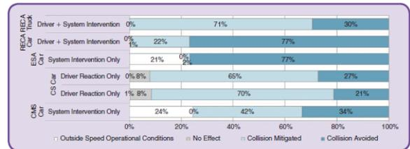
Figure 6. Results of SIMPATO assessment for rear end collisions by ADAS and safety systems (SIMPATO, 2015)
