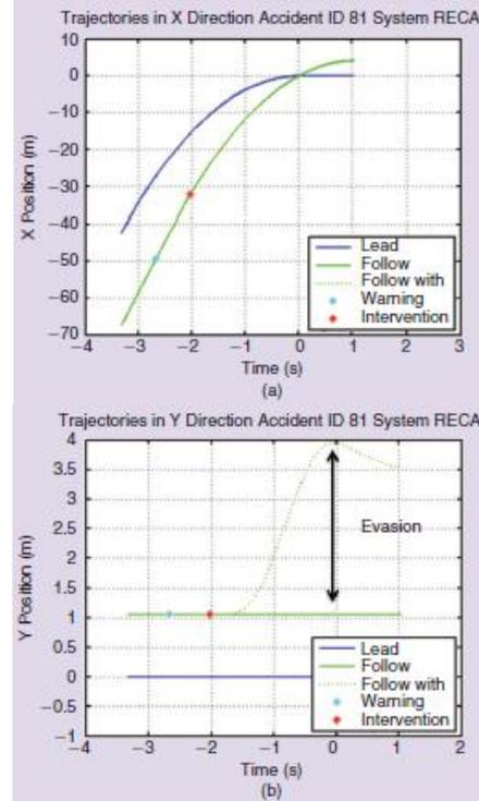
Figure 5 Results of for a rear-end collision situation without and with RECA taken from (SIMPATO, 2015)
